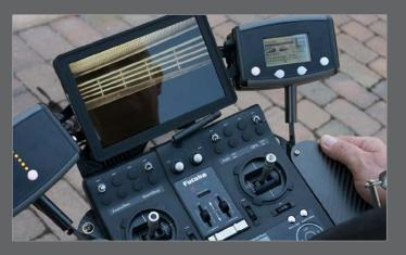
View real-time data on the monitor of the Mobile Ground Station or using the video goggles. Freely adjust the Falcon 8's alignment and image zoom using the live image.
