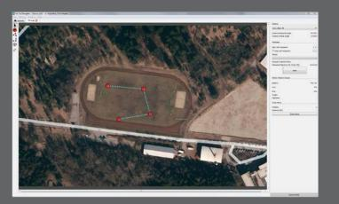
Flight planning is simple, much is contained in the Mobile Ground Station firmware. Simply enter your required parameters to survey your area of interest right at the project site. Flight pattern and attitude are automatically optimized and defined by your settings.
