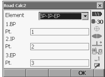
4. Input the point number of BP point (reference point), IP point and EP point then press **[OK]**
