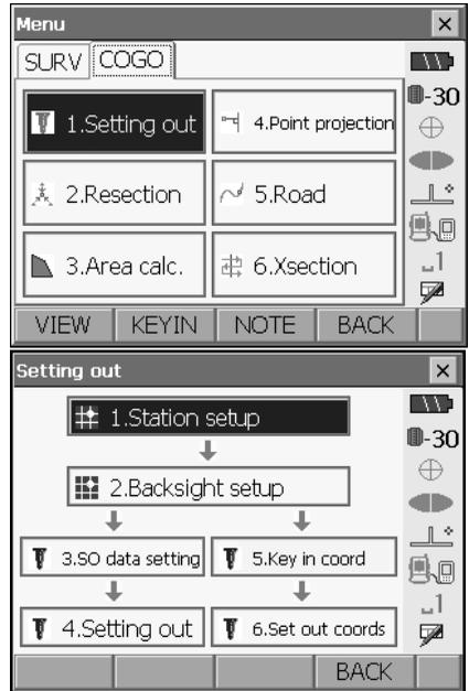
2. Select "Station setup" to display <Station setup>. Enter data for the instrument station and press **[OK]** to move to Backsight setup.
