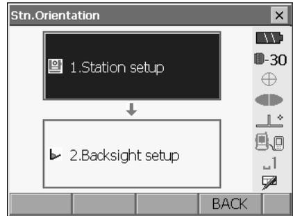
4. Select "Backsight setup" in <Stn. Orientation> and enter backsight station data.
