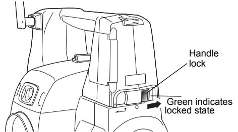
2. Pull the lock levers towards you and slide the handle back and up to remove. The handle lock levers, once released, will return to the original position.
