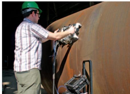
HSMT-Flex scanner used for TOFD applications (PV-100).
