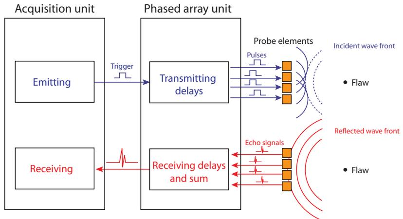
To generate a beam, the various probe elements are pulsed at slightly different times. By precisely controlling the delays between the probe elements, beams of various angles, focal distances, and focal spot sizes can be produced. The echo from the desired focal point hits the various transducer elements with a computable time shift. The signals received at each transducer element are time-shifted before being summed together.
