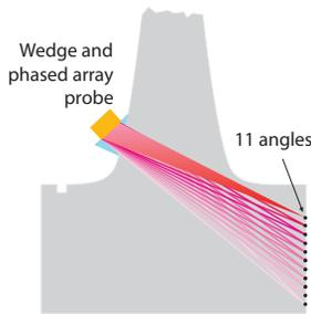
Multiple-angle inspection with one multielement probe.
