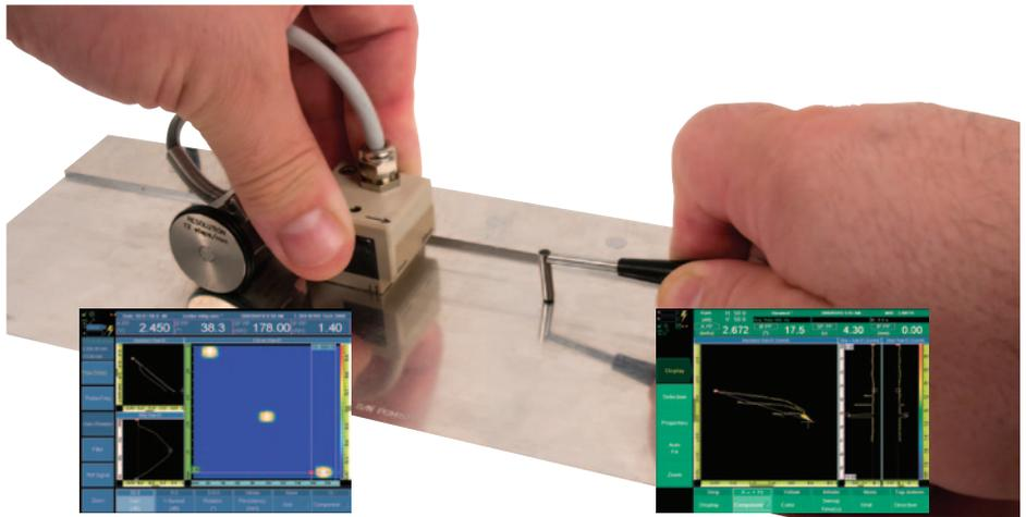
Eddy current array probes can replace one axis of a two-axis scan and offer greater flexibility in the eddy current setup.
