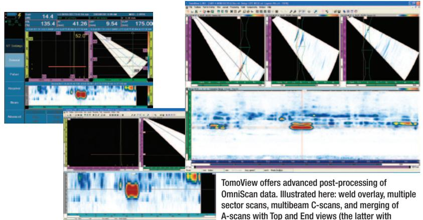
TomoView offers advanced post-processing of OmniScan data. Illustrated here: weld overlay, multiple sector scans, multibeam C-scans, and merging of A-scans with Top and End views (the latter with rebound display).
