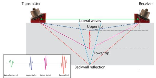
General view of TOFD setup for linear weld inspection showing lateral wave, backwall echo, and diffracted signals on the A-scan.
