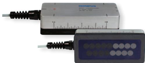
Transmit-receive probe for corrosion detection down to 6 mm (0.25 in.) in aluminum
