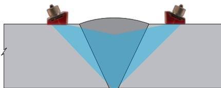
Weld inspection using TOFD.
