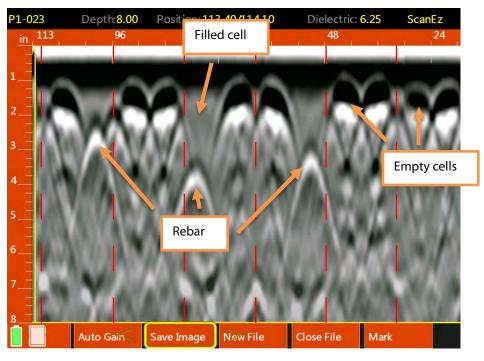
and thus no reflection is produced. Each of the filled cells has a rebar as reinforcement. Those show as the hyperbolas in the filled cells.
