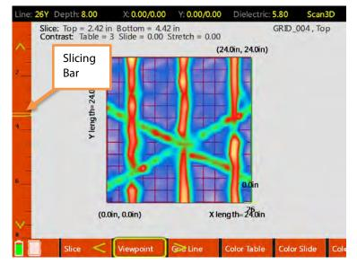
**Grid Line:** Toggles to the individual lines in the grid which are then viewed in the 2D linescan and the oblique 3D views. The currently selected line is noted at the top-left corner of the screen.
